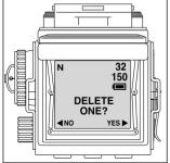
Press Image delete button once and DELETE ONE? sign appears in the center of the monitor accompanied by < NO YES > below it. Press Right button to delete the image and Left to cancel deletion, returning to Playback mode.
